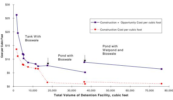
Figure III-1: Detention Facility Costs per Cubic Foot Detention Volume Required
